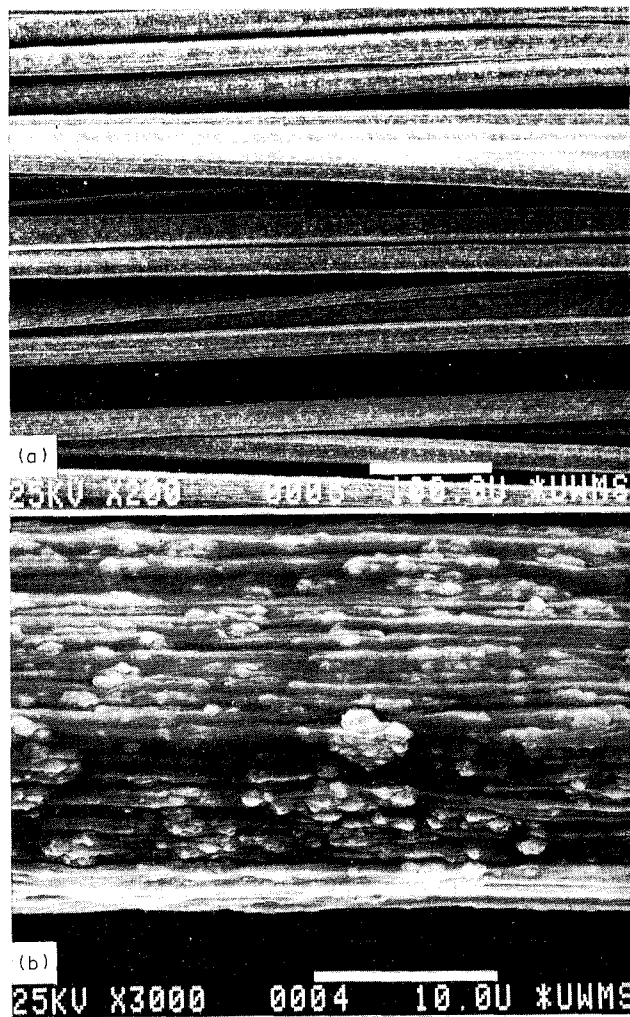
Fig. 9. (a) SEM image of several Nb-Ti filaments from 0.622 mm wire after acid removal of Cu matrix, (b) SEM image of filament surface from 0.622 mm wire.
